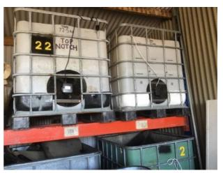
For hoppers they have developed a system that both carries and dries the nuts, made from a standard agricultural cube container with the top cut out and a bottom trapdoor-controlled chute and a fan that blows air through the nuts. These affordable hoppers can take half a tonne of nuts.
